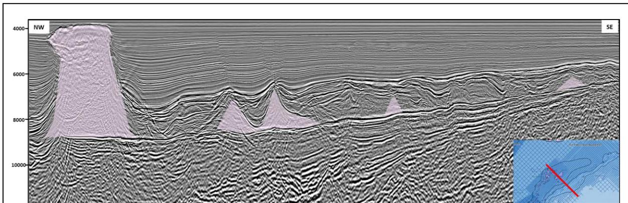
Figure 2: RTM depth stack shows improved image in presalt and postsalt sediments, salt diapir observed in west central Yucatan basin.
