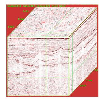
Figure 8: 3D interpolated traces using the 3D geological time model and 2D Cube methodology described in this paper.
