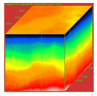
Figure 7: 3D geological time model which are used to interpolate a 3D demigrated seismic traces.
