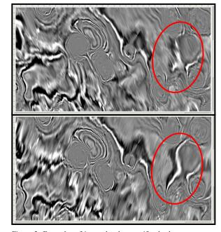
Figure 3: Examples of interpolated traces if only those traces on certain azimuthal searching orientation are used. A) along -20 degrees; B) along +20 degrees (close to the strike direction)
