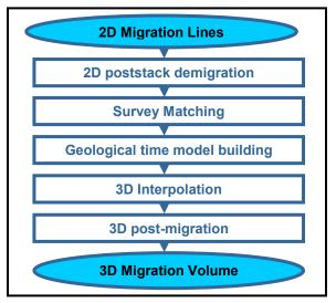
Figure1: Workflow diagram for 2DCube technology
