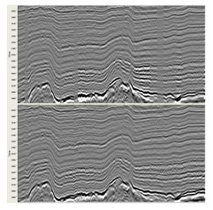
Figure 4: 2D demigrated zigzag section - A) Before and B) After survey matching and automatic intersection tying
