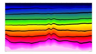
Figure 6: 2D geological time model which ties at all intersections between 2D lines. The line shown here is the same as shown in Figure 5. The Model layering closely matches the geology.
