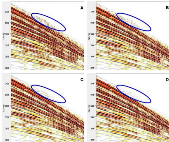
Figure 6: CFP redatuming data regularization for different intermediate receiver grid sizes: 17.5m (A); 15.0m (B); 12.5m(C); and 10.0m (D). Notice the aliasing noise within the blue circles.
