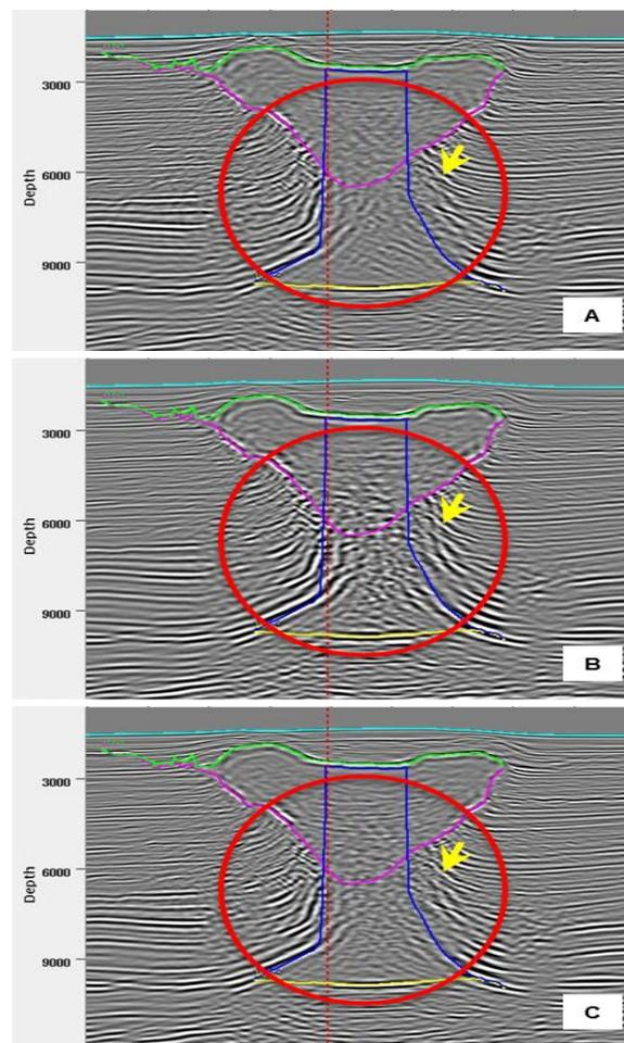
Figure 8: (A) The RTM image of weighted summing Kepler and Justice Surveys' RTM images. (B) The RTM image for redatuming data regularization input with large aperture. (C) The RTM image for redatuming data regularization input with small aperture.
