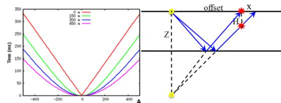
Figure 3: Diagram to show the redatuming depth determination. (A) The CFP operator kinematic with different redatuming depth. (B) CFP aperture definition related to redatuming depth.
