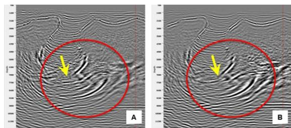
Figure 9: (A) The RTM image of weighted summing Kepler and Justice surveys' RTM images. (B) The RTM image for redatuming data regularization input. More complex salt model may be needed within the red circle area.
