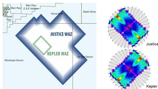
Figure 1: Map shows the location of the Justice and Kepler WAZ surveys on the left. The corresponding surface azimuth coverage is shown on the right.
