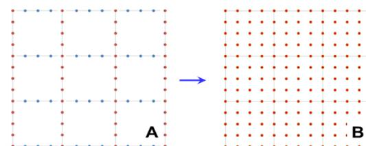
Figure 4: After shot regularization, the shot spacing changes from 150mx600m and 600mx150m (A) to 150mx150m shot spacing (B).
