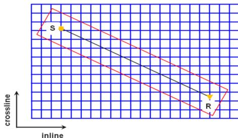
Figure 2: The aperture is defined differently for each receiver. For output source-receiver (S-R), the aperture is defined as the red rectangle. Then aperture is divided into calculation grids (blue) which are oriented along the inline and crossline directions.
