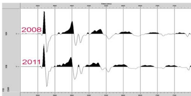
Figure 3: Hydrophone measurements from a selected receiver station from 2008 (upper) and 2011 (lower). The shots are from the closest offsets of a 100 cu. inch gun
