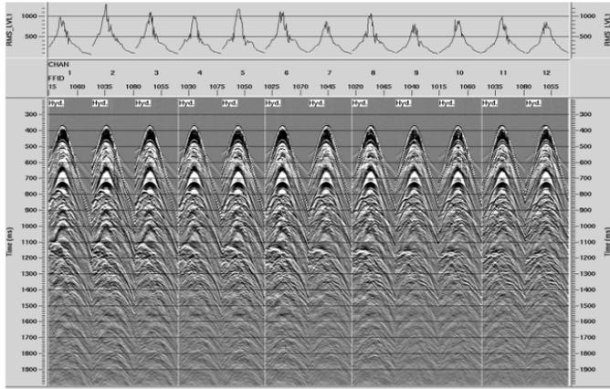
Figure 4: Hydrophone CRGs of 2006 cu.in. source array of all receiver stations from 2011
