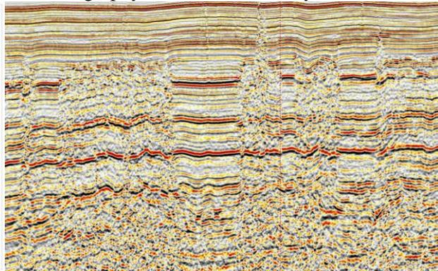
**Figure 2:** Without correct karst velocity model, the sub-karst images are often poor and non-geological.
