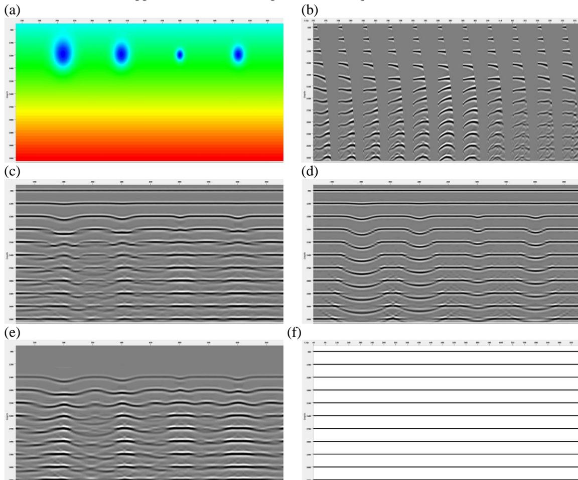
**Figure 3:** Synthetic examples. (a) True velocity model for synthetic data. Migration results for smooth background velocity: (b) CIGs around the low velocity anomaly on far left; (c) full stack; (d) near offset stack; (e) far offset stack. Three stacks (c-e) show very different images. (f) true reflectivity model.
