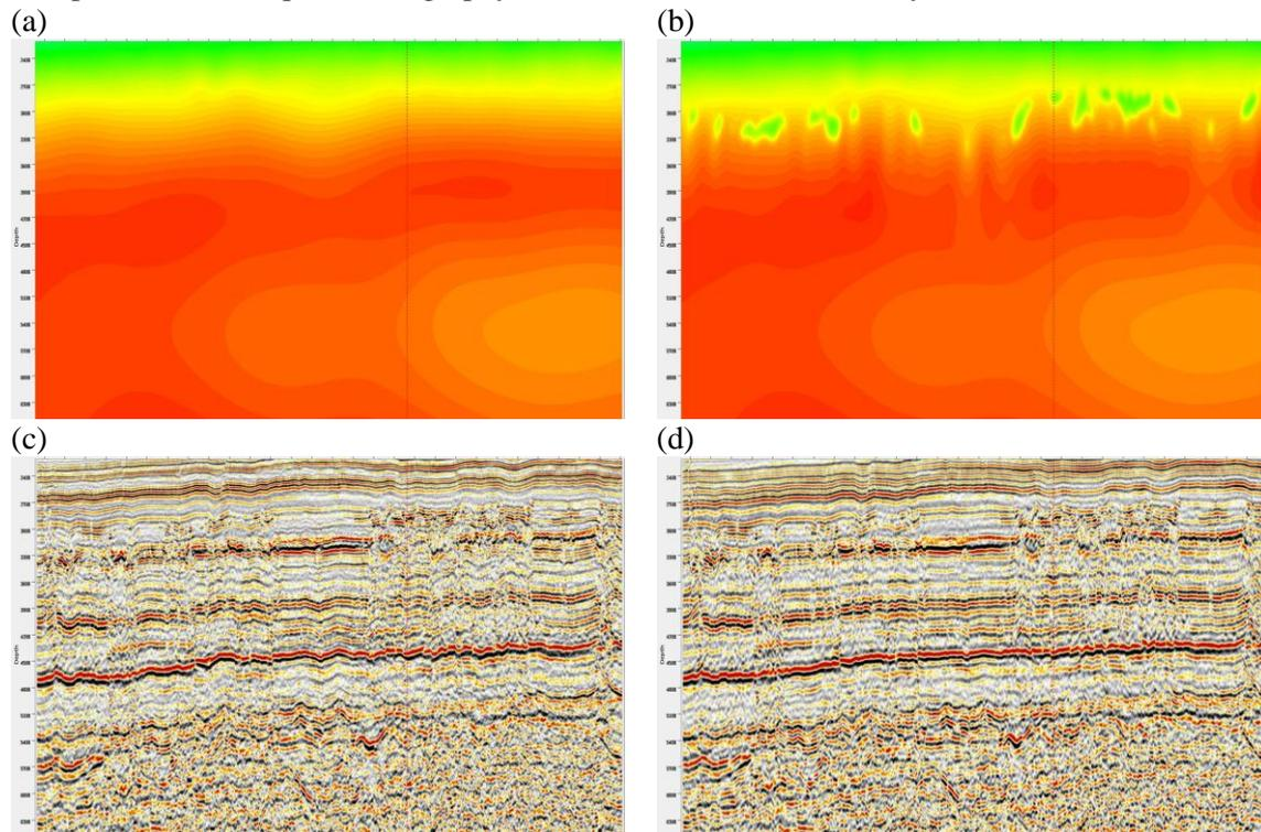
**Figure 6:** Velocity model update and corresponding near offset stack responses. (a) Velocity models before (a) and after (b) karst modelling and horizon driven tomography. (c) Migration near offset stack with velocity model shown in (a). (d) Migration near offset stack with updated velocity model shown in (b).
