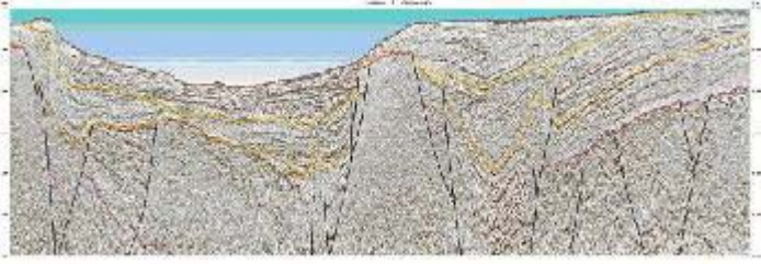
Fig 2: 600 km long seismic line acquired from the Canadian coast to the Greenland coast. The line shows deep basins and rift systems in Paleozoic, Mesozoic and younger sediments.
