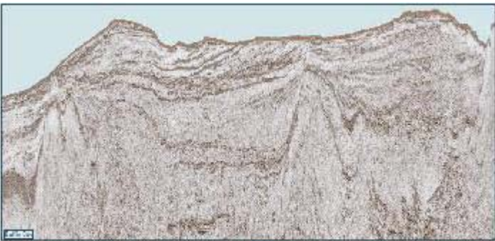
Fig 3: Seismic line in the Baffin Bay demonstrate large traps and deep basins.
