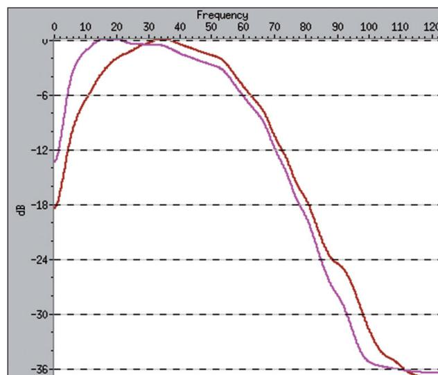
Figure 4 Amplitude spectrum of the shot gathers shown in Figure 3 in a window below top basalt; the pink line shows the enhanced low frequency content after application of the matching operator and brown line without.
