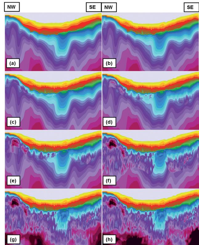
Figure 10 Tomographic updates: (a) iteration 0 – reference model derived from full sequence migration multi-velocity analysis stacking velocities; (b) update through Tertiary; (c) update to Flett formation and top Palaeocene; (d) update to Lamba formation; (e) update to Vailla formation; (f) update to Sullom formation; (g) update to Top Triassic; (h) final update for late Mesozoic and Palaeozoic.
