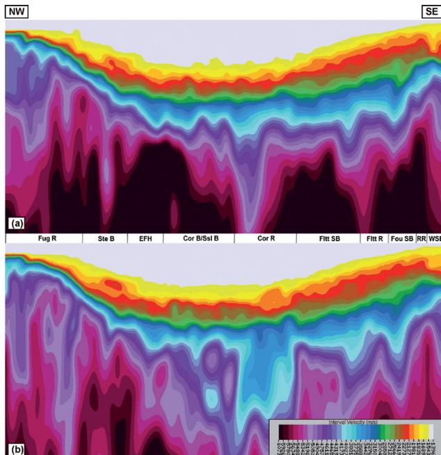
**Figure 8** Final time migration interval velocity fields (a) derived from the original processing and (b) from reprocessing with the inclusion of full sequence migration multi-velocity analysis. A significant reduction of velocity is observed in the vicinity of the Corona Ridge. Annotated features refer to those described in Figure 7.
