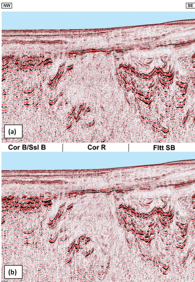
Figure 9 Initial (iteration 0) pre-stack Kirchhoff depth migration image obtained from (a) velocities derived from the original time processing and (b) from the reprocessing with reference to Figure 10(a). The input dataset in both examples is identical. Annotated features refer to those given in Figure 7.
