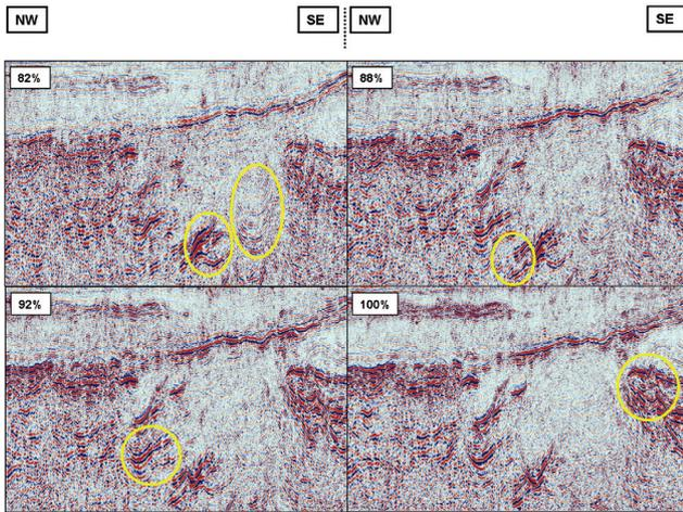
**Figure 5** Zoom of selected full sequence migration multi-velocity analysis panels across the northern Corona Ridge with the percentage velocity variation relative to the initial 100% function annotated. Examples of preferred images are ringed.
