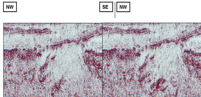
**Figure 6** Initial 2D Kirchhoff pre-stack time migration image from the initial (100%) reference function (left) and updated image (right) after re-migrating and stacking with the derived full sequence migration multi-velocity analysis function.
