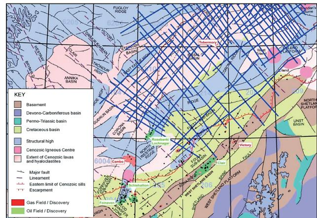
Figure 2 Tectonic elements map of the Faroe-Shetland Basin modified from Moy (2010) showing the FSB 1999/2000 2D survey lines in dark blue, wells in black and oil/gas discoveries.
