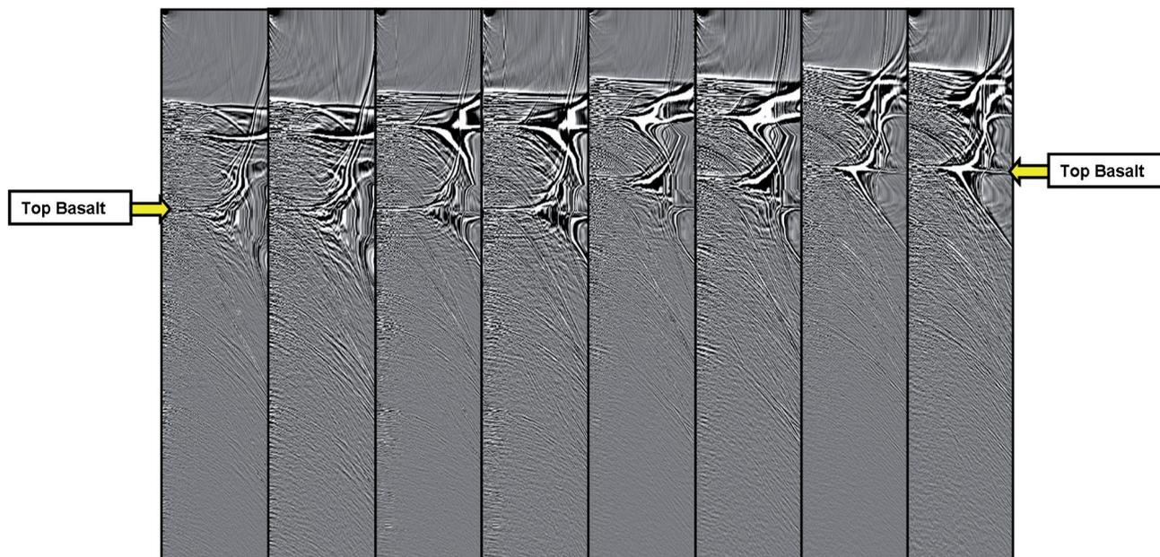
Figure 3 Selected shot gathers sampling the extensive Palaeogene flood basalts in the northwestern part of the FSB 1999 survey area. Gathers are shown side-by-side before and after application of the low frequency boosting operator.
