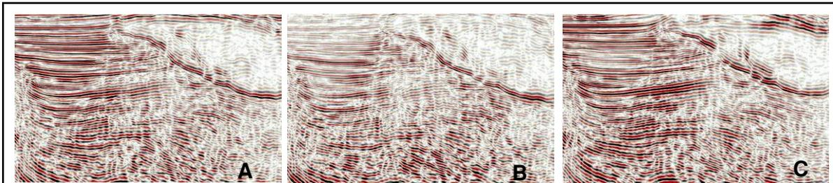
Figure 2: An example of DIT scan panels with delayed imaging time: A) 0 ms; B) + 100 ms; C) - 100 ms
