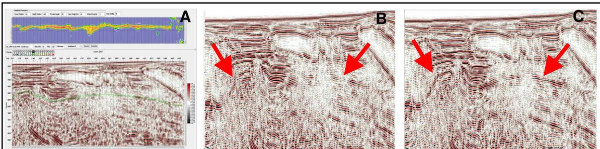
Figure 3: A) DIT scan picking interface; B) Regular RTM image using initial velocity model; C) Composite RTM image using the same initial velocity model as Figure B, after DIT scan
