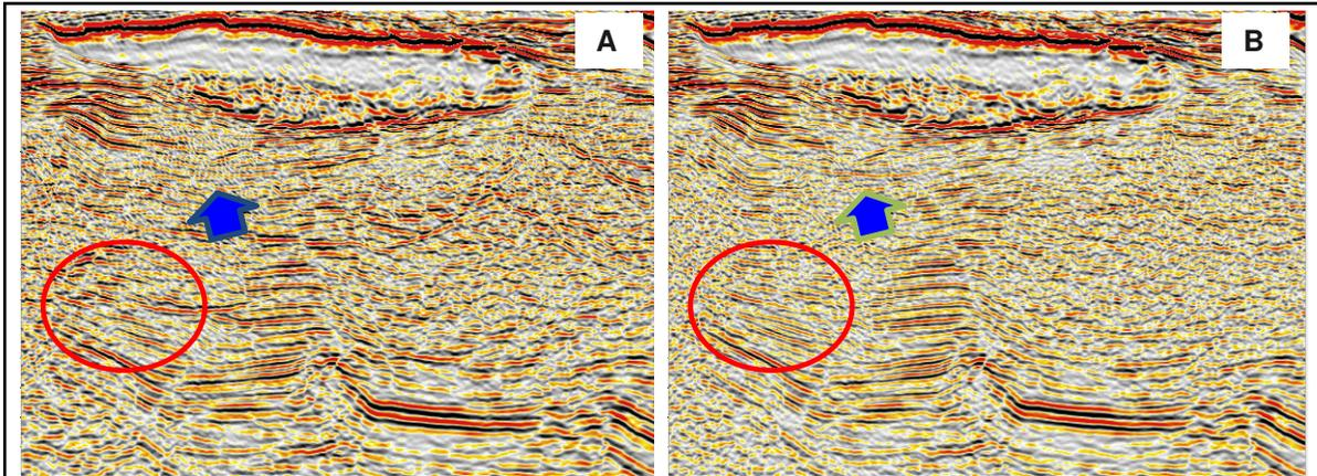
Figure 1: A) Single sequence RTM image without SRME; B) Single sequence RTM image with 3D true azimuth SRME
