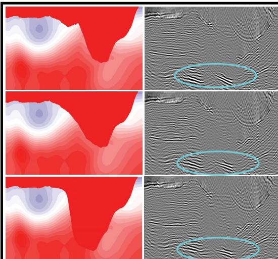
**Figure 6:** Left column shows different salt interpretations and velocity models; Right column shows the corresponding layer-stripping RTM images using the velocity models on the left.
