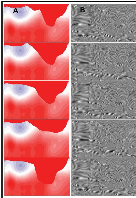
**Figure 2:** A) Corresponding salt interpretation and velocity models; B) beam migration images;
