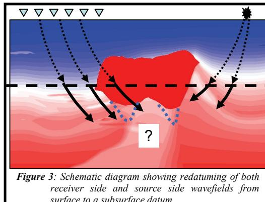
**Figure 3:** Schematic diagram showing redatuming of both receiver side and source side wavefields from surface to a subsurface datum.
