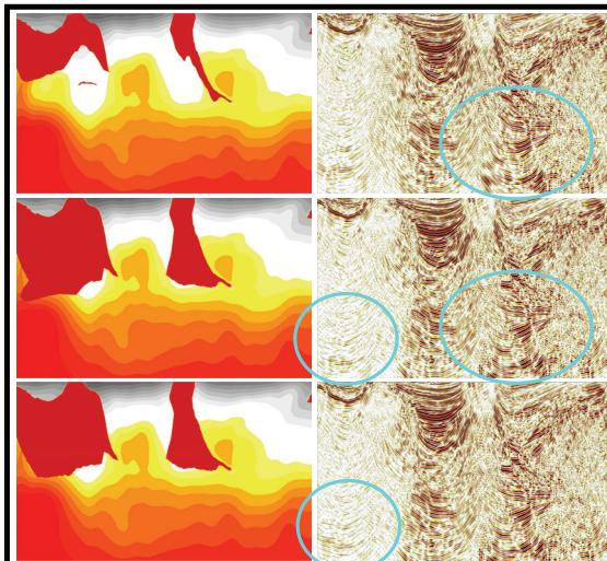
**Figure 7:** Left column shows different salt interpretations and velocity models; Right column shows the corresponding layer-stripping RTM images using the velocity models on the left.
