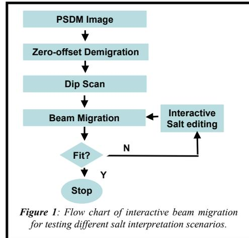
Figure 1: Flow chart of interactive beam migration for testing different salt interpretation scenarios.
