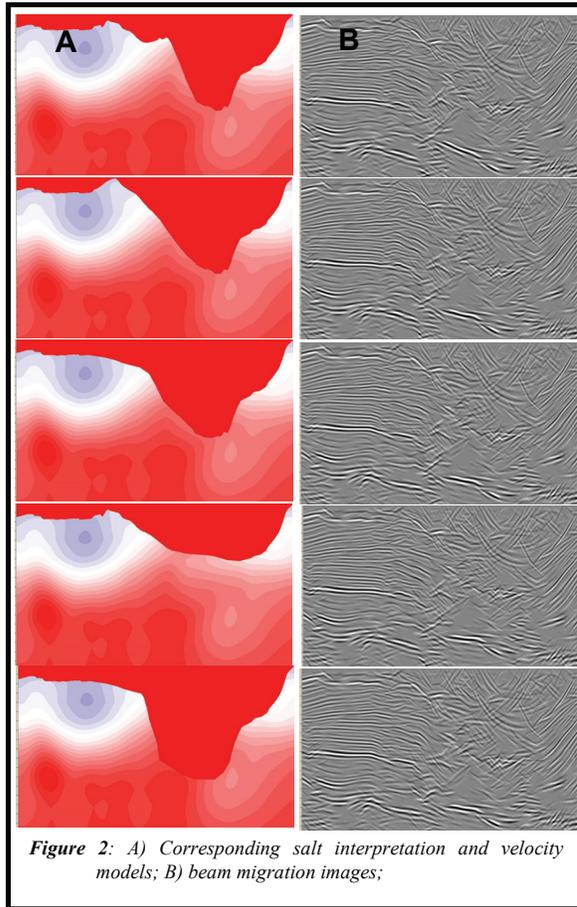
Figure 2: A) Corresponding salt interpretation and velocity models; B) beam migration images;
