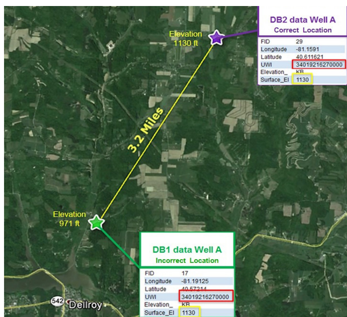
Figure 2. Example of surface well spot correction for validated well headers. Two databases list the same well UWI with different locations. In this case surface elevation data helped confirm the DB2 database entry was correct.
