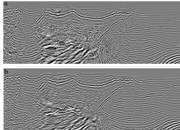
**Figure 10.** Final VTI RTM results from the combined Kepler and Justice processing, showing a) Kepler, and b) Justice.
