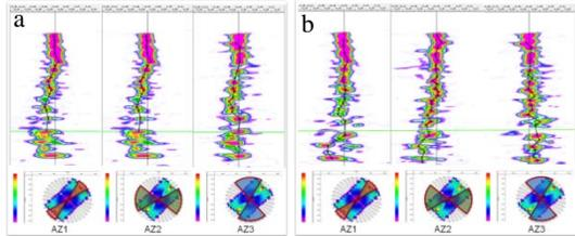
**Figure 7.** Semblance displays from Kepler three azimuth-sector tomography a) prior to tomography, and b) after one pass of azimuth-sector tomography.
