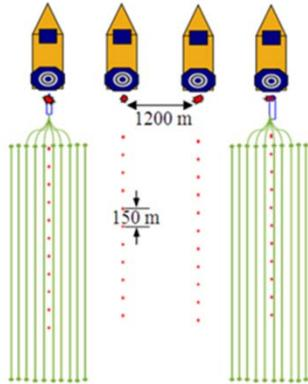
**Figure 2.** Acquisition set up for the Kepler and Justice surveys.
