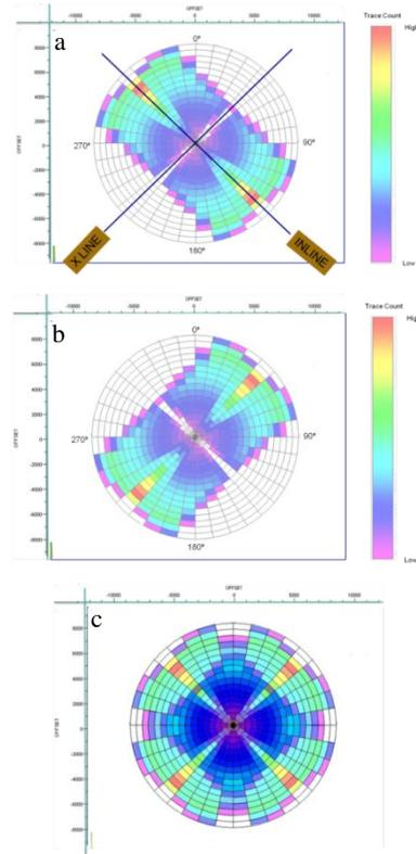
**Figure 4.** A series of Rose diagrams showing the azimuth and offset distribution for a) the Justice survey; b) the Kepler survey; c) the Justice and Kepler surveys combined.
