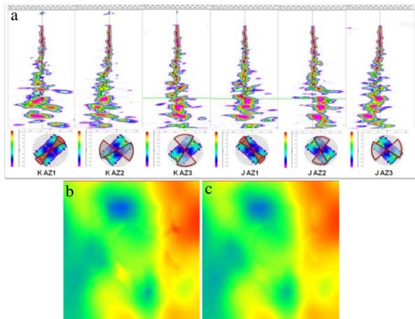
**Figure 8.** Kepler plus Justice three azimuth tomography: a) semblance display after tomography, same location as Figure 7, b) 3600 m velocity depth slice after tomography using the Kepler survey only, c) 3600 m depth slice after tomography using Kepler plus Justice.
