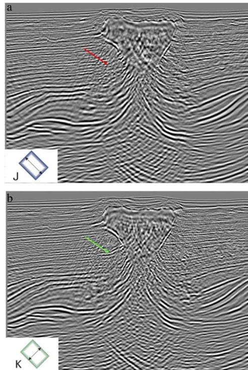
**Figure 6.** Crossline direction: VTI RTM of a) the Justice survey and b) the Kepler survey. Green and red markers indicate areas of good and poor imaging, respectively.
