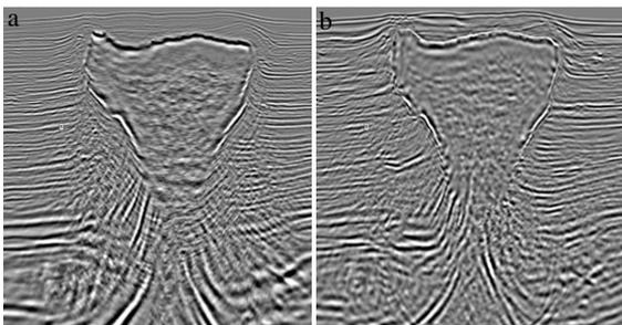
**Figure 9.** Final migration results from the Kepler only processing, showing a) VTI Kirchhoff PSDM and b) VTI RTM.
