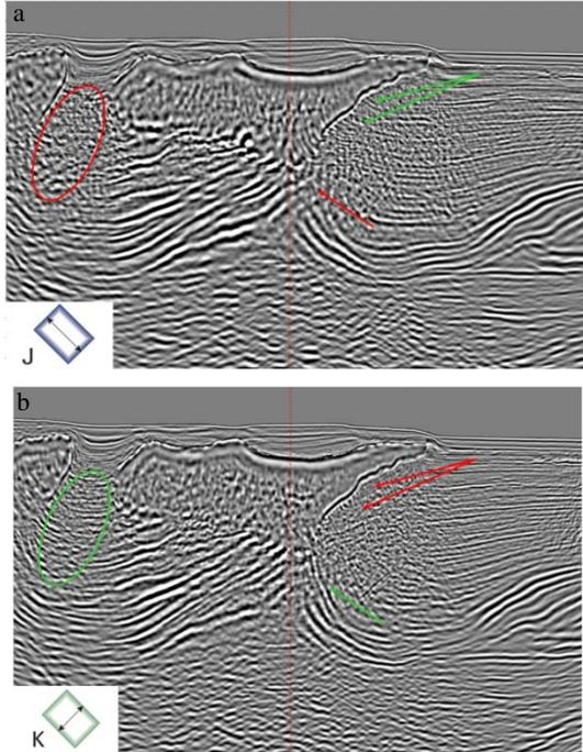
**Figure 5.** Inline direction: VTI RTM of a) the Justice survey and b) the Kepler survey. Green and red markers indicate areas of good and poor imaging, respectively.
