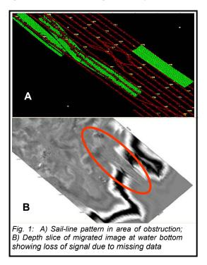
The WAZ method naturally lends itself to undershooting obstructions to cover longer offsets and wider azimuths but it is at a disadvantage when acquiring near offset data near obstructions. Figure 1A shows the pattern of shots and cables in the area of production platforms from WAZ survey and Figure 1B shows the effect of the missing data on a depth slice that intersects the water bottom.
