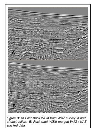
The resulting stack volumes are input to the post-stack WEM to generate the reflectivity model for WFE multiple prediction. When comparing the two 3D migrated images we see significant improvement in continuity and resolution as well as a more stable wavelet in the shallow multiple generating section. All these enhancements will
