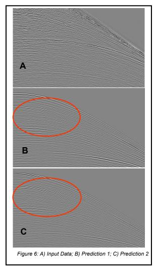
The quality of the multiple prediction is largely dependent upon the integrity of the reflectivity model. We try to match as closely as possible the wavelet and resolution of the input shot data. This contributes to a better prediction and allows a more conservative approach to the subtraction which is less likely to adversely effect primary reflections.
