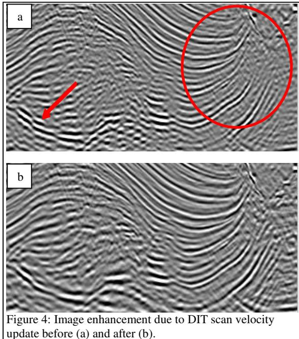
Figure 4: Image enhancement due to DIT scan velocity update before (a) and after (b).
