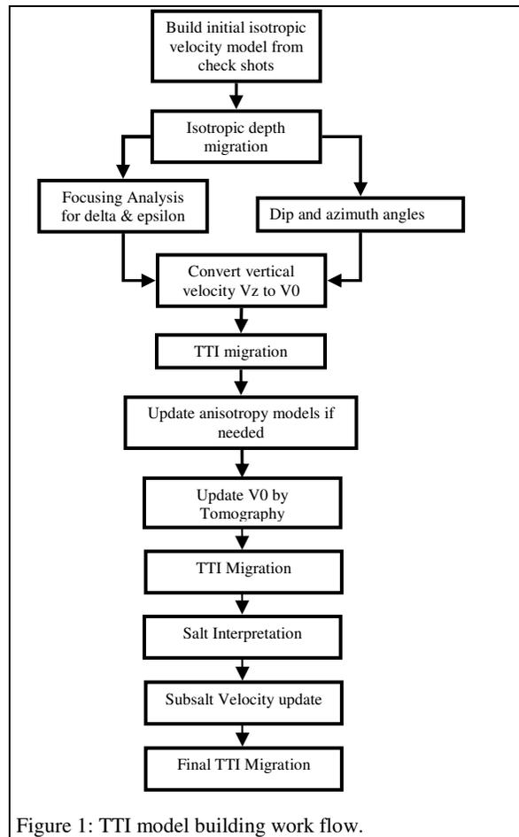
Figure 1: TTI model building work flow.
