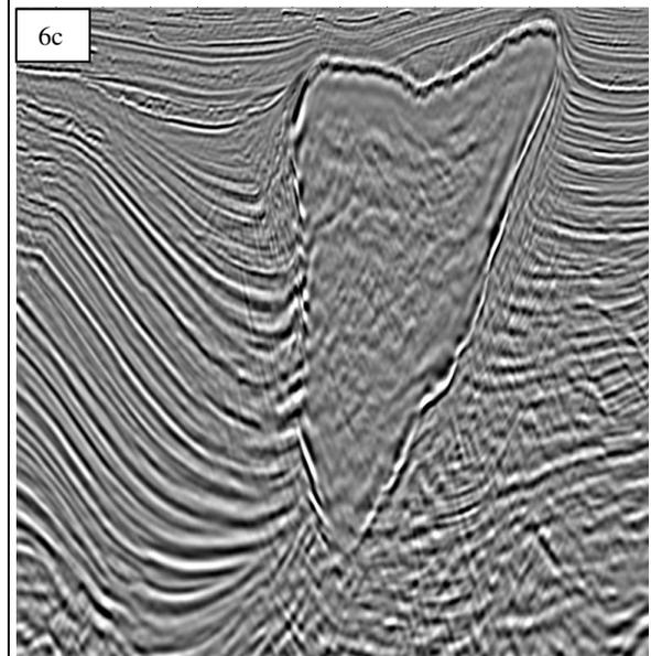
Figure 6: Inline comparisons of (a) VTI Kirchhoff, (b) TTI Kirchhoff and (c) TTI RTM PSDMs over a complex salt body. Note the improvements in salt body geometry, overhangs and the subsalt reflections in TTI RTM section.
