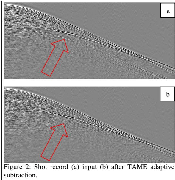
Figure 2: Shot record (a) input (b) after TAME adaptive subtraction.
