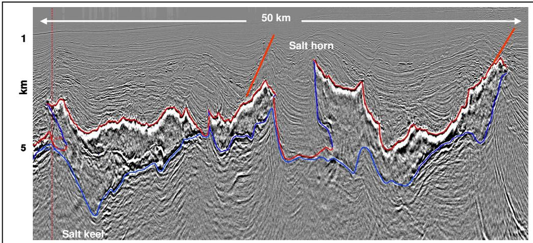
Figure 1: A north (left)-south (right) seismic section in western Mississippi Canyon area (water depth < 1km) shows two interesting features, salt horns on top of salt and salt keels in the base of salt level, which are most likely under regional structural control. Upthrown strata against the base of salt can be of economic potentials.
