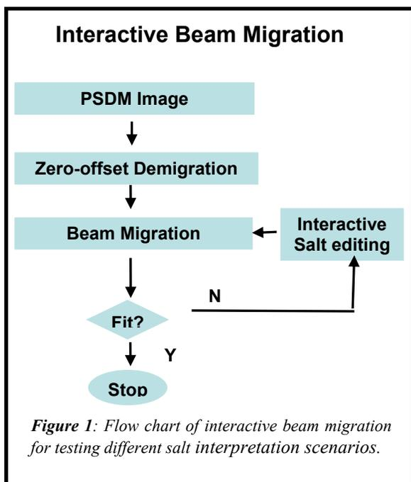
Figure 1: Flow chart of interactive beam migration for testing different salt interpretation scenarios.
